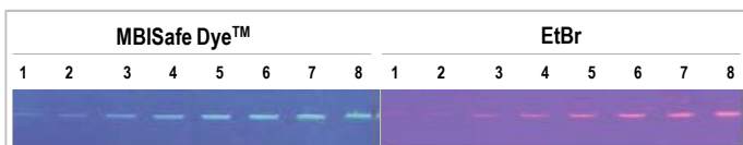
Fig. 3. Gel analysis of serial diluted genomic DNA using MBISafe Dye™ Nucleic Acid Staining Solution (20,000x) and EtBr
