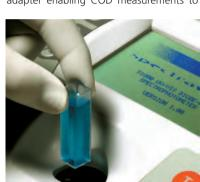
be made using standard 16mm diameter test tubes plus the cell holder may be removed for cleaning. Another version of the instrument, the WPA S1200T, is available with a factory fitted electrically heated cell holder for thermostatted measurements at 37°C.
