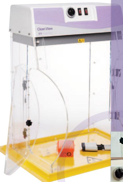
UV Sterilisation Cabinets provide a convenient area for setting up PCR reactions in a nucleic acid free environment
