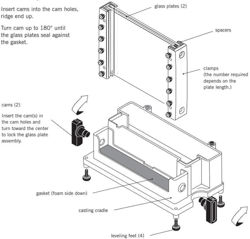
**Note:** It is easier to keep the caster balanced if you turn both cams toward the center of the caster.
