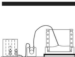
**Fig 6.** Pouring a gradient gel.
