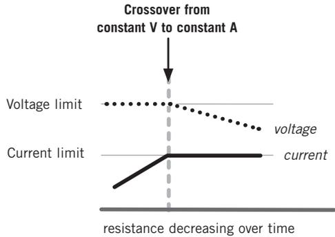
There are some conditions when the power supply will operate at the upper limit of 150 W of constant power. When this occurs, both the constant V and the constant mA lights will be lit at the same time.
