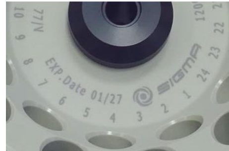
Fig. 4: Different service life – engraving on the bucket/rotor
