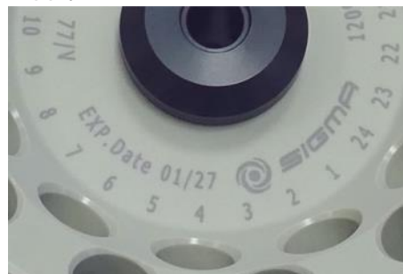
Fig. 5: Different service life – engraving on the bucket/rotor
