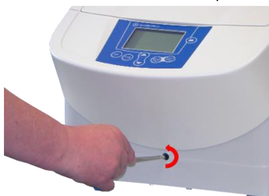
Fig. 11: Manual release of the lid lock
