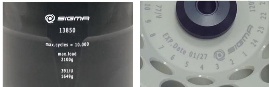
Fig. 4: Different service life – engraving on the bucket/rotor
