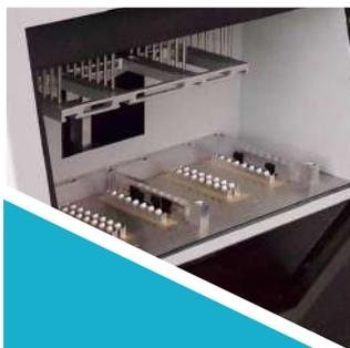
**Sample injection:** Adapting to the automation equipment of various companies, the samples can be directly placed in the sample bin of the automatic equipment in multiples, eliminating the tedious work of placing samples multiple times.
