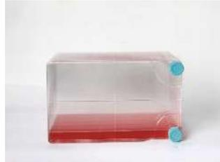
Lay the cell factory on its side to balance the liquid level.
