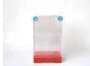
With the liquid-adding opening upward, the culture medium will be evenly distributed to each layer after standing.
