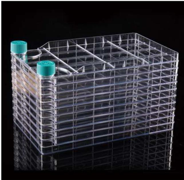
NEST BioFactory™ system is a well-designed cell culture device that utilizes the maximum culture area in a limited space, saving a large amount of space, low-cost to achieve the purpose of expanding production capacity.
