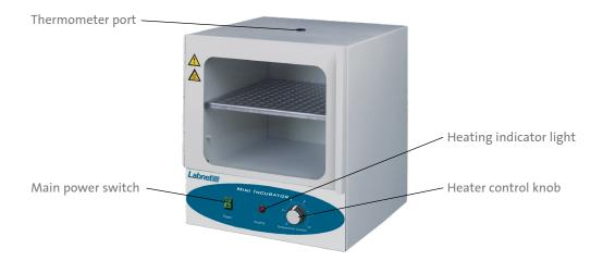
Install the shelf at the desired height, shelf edges down. If you intend to place samples on the bottom of the chamber, install the shelf so that it sits edges down on the chamber bottom, thus creating an air gap between the chamber bottom and your samples.
