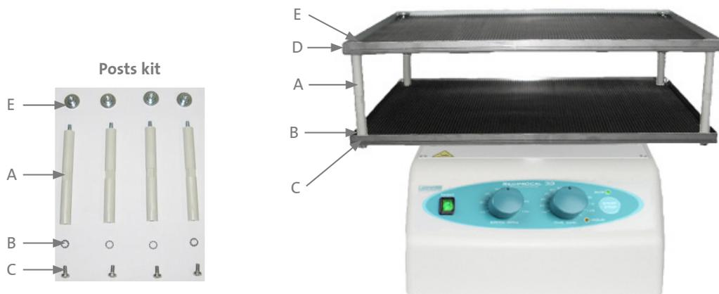
1. Set the four posts (A) above the four holes at the corners of the bottom platform.
