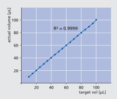
JET injectors enable the injection of liquids with an accuracy and precision exceeding 98 % over the entire volume range
