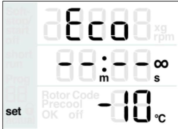
Fig. 10: Indication of the Eco mode and speed value in alternation
