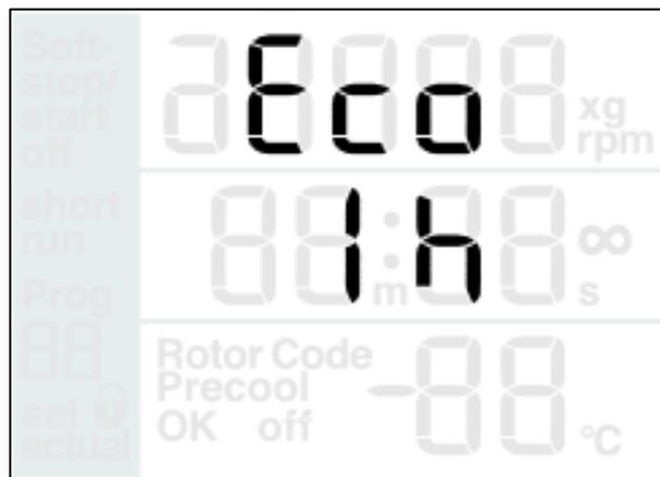
Fig. 11: Adjusting the turn-off time
