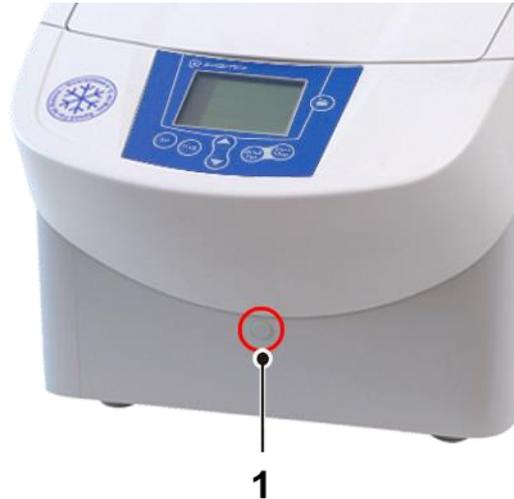
Fig. 13: Position of the opening for the emergency lid release
