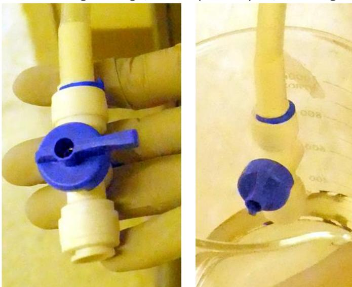
6. Making sure the stopcocks on the drainage tubes are in the closed position (i.e., not in-line with the axis of the tube, but turned perpendicular to it), open reservoirs A/left & B/right and pour 500 mL of deionized water into each reservoir opening, re-securing the reservoir lids when finished. A small piece of cotton is pre-installed in the ventilation hole of each reservoir lid to minimize bubbles rising out of the chamber and should be replaced when needed.
