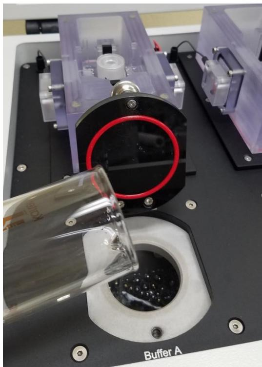
7. Wash the system for 15 minutes by turning on the pumps for both reservoirs A & B (see description of SmartBox User Interface (UI) below in the Operation section of the manual).
